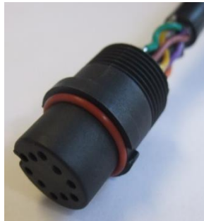
Figure 15 O-Ring over Connector Body
