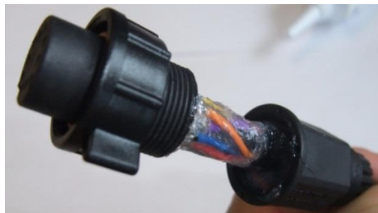
Figure 17 Silicone in the Grommet
